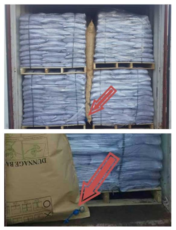
The coating, inflated paper bag and the blue ball that the red arrow points to are all used for quakeproof, which help the products be intact.
